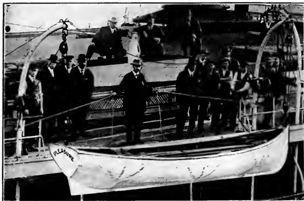
One man lowering lifeboat from deck. He can control the windlass from the lifeboat just as easily. See below.
